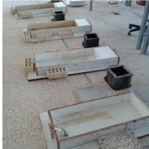
Fig. 4a Wooden moulds before casting
