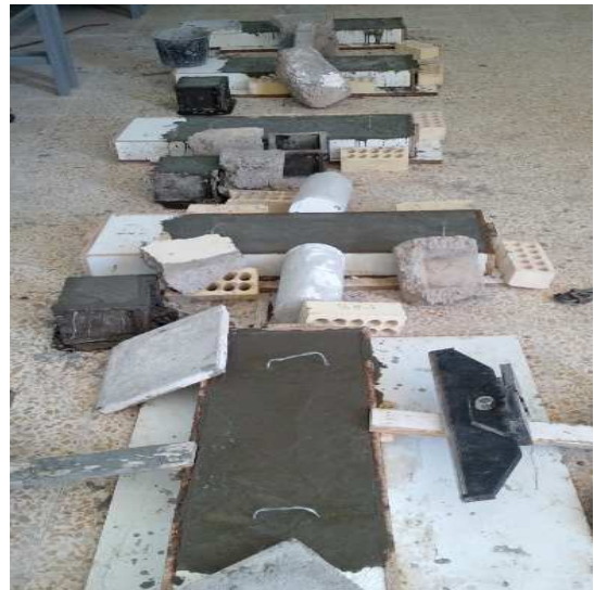
Fig. 4b Concrete wide beams after casting
