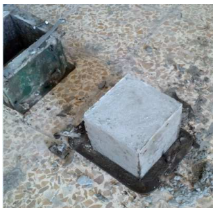
Fig. 3. Concrete cube for compression test
